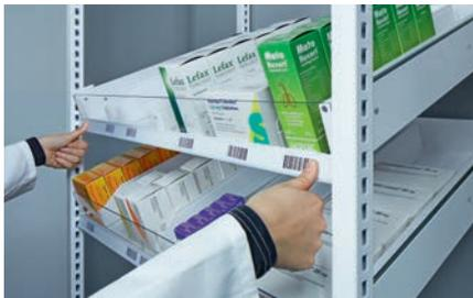
**Touch Release:** the Touch Release mechanism ensures the simple and safe opening of the sloping trays. By slightly pushing against the sloping tray on both sides of the handle bar the safety mechanism is released and the sloping tray moves out. When pushing the tray back in, a clicking sound confirms that it is safely locked in closed position.
