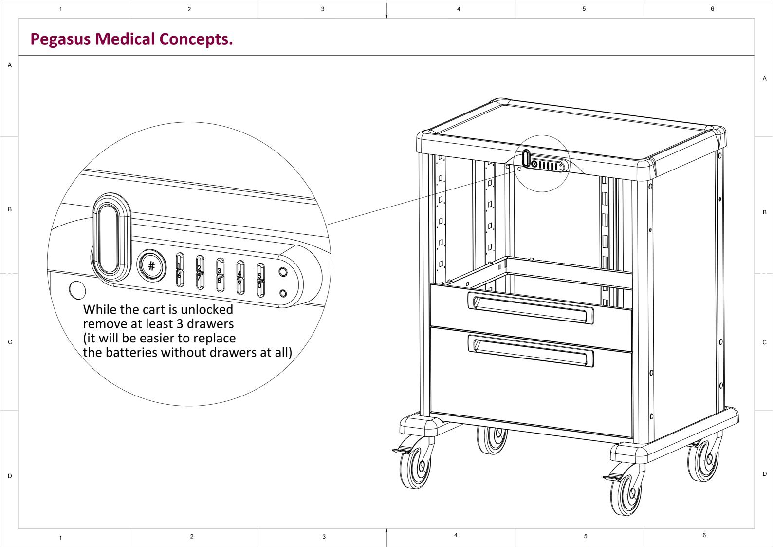
On every drawer's side, you'll see a grey plastic tab in the telescopic rail. Push the tab toward the free side on both telescopic sliders (the directions are opposite) and pull the drawer outside (while holding the tabs).
